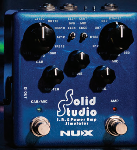
IR Loader with built-in cabinet, microphones and microphone positions, power amp simulator with 3 tubes, power amp controls
